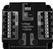
**VRM:** The voltage regulator module regulates the voltage of the electricity that travels to any cameras or sensors on the robot, as well as the radio.
