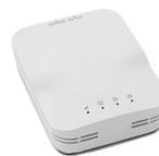
**Radio:** Puts out a WiFi signal to connect to the driver station laptop, so that the drive team can control the robot.
