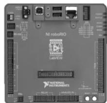
**roboRIO:** The roboRIO is the 'brain' of the robot and stores all of the robot's code, controlling the amount of power sent from the PDP to other components.
